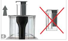
When whisking egg whites or whipping cream, remove the double pusher from the feed tube to allow more air in.
