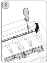
Unscrew retaining plates either side of the element. Lift up to remove the plate.
