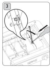
Unscrew brass links and wires using a 6mm spanner and screw driver.
