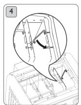
Bend brass links and wires away from the element.
