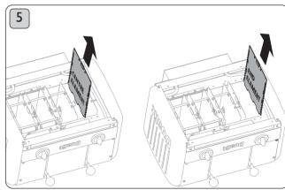
Remove element. To re-assemble, reverse procedure ensuring wires and parts are correctly positioned. Ensure new element is marked the same as the one removed and is seated correctly in the channels either side. PAT test before use.
