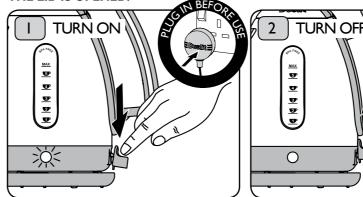
Plug the kettle into the power socket. Press the 'On/Off' switch down. The power LED will illuminate and the kettle will start to heat up. If the kettle is accidentally switched on with no water inside, the boil-dry device will switch off the heating element to prevent damage to the kettle.
