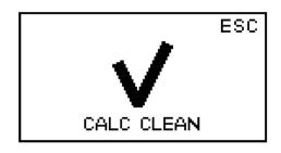
Press the "Cappuccino" button to exit the descaling cycle.
