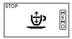
When the "STOP" icon is displayed, press the "Espresso" button as soon as the desired amount of coffee is reached.
