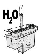
When filling the water tank, use sterile disposable gloves to prevent bacteriological contamination
