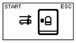
The machine reminds you to install the water dispensing spout. Check that the water dispensing spout is correctly installed. Press the "Espresso" button to confirm. The machine starts dispensing hot water.
