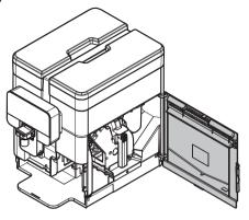
Close the door again and brew I-2 cups of coffee to verify the changes in the grinding degree. Repeat the procedure until you reach the desired grind setting. The reference marks indicate the grind setting. There are different grind settings to choose from with the following references:
