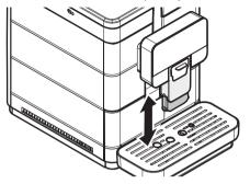
Manually move the dispensing spout up or down to adjust its height.
