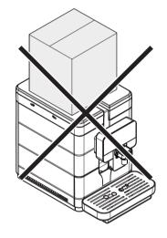
Due to the total weight, do not stack more than three machines on top of each other. The machine should be stored in its original packaging, in a dry and/or dust-FREE place.
