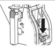
Make sure that the hook which locks the brew group is in the correct position. firmly press the "PRESS" button to check its position.
