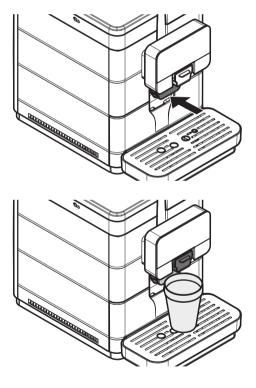
Before brewing any product and/or when bringing the dispensing spout back to its normal position, ensure that it is correctly positioned. This can be evidenced by the CLICK indicating correct positioning.
