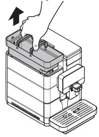
Rinse and fill it with fresh water; do not exceed the level (MAX) indicated on the tank.
