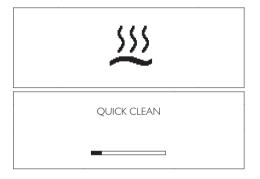
In this case, the washing cycle is performed with hot water only and the suction tube is not used. At the end of the cleaning cycle, it must be compulsorily washed under running water. Wait until the cycle stops automatically. The machine will go back to the ready for use state.
