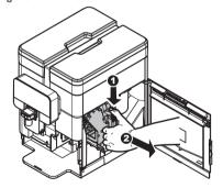
Press the "OK" button to confirm the removal of the brew
