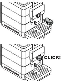
Before using the Cappuccinatore, clean it as described in the "Cleaning the Cappuccinatore (After Each Use)" section.
