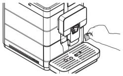
Insert the Cappuccinatore into its seat until it locks into place. Check that it cannot be pulled out.
