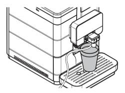
Select "OK" and press the "OK" button. The machine dispenses a quantity of water sufficient to rinse the milk circuit. The following screens are displayed:
