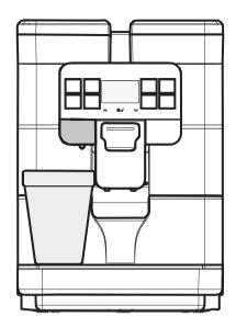
Press the "Hot Water" button to start dispensing HOT WATER.
