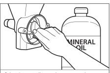
If the Grain Mill Attachment is to be stored for a long period of time, lightly coat the burrs with mineral oil. Before next use, hand wash as directed in the "Before first use" section to remove the mineral oil.
